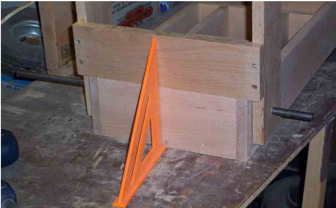
Attaching the bottom horizontal support to the gun rack
